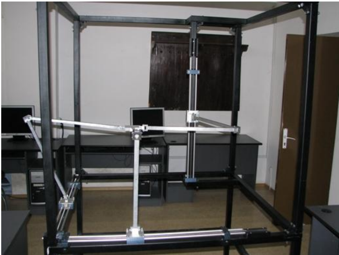
ISOGLIDE parallel robot realized at Dept. of Mechatronics, TU Cluj-Napoca, Romania
